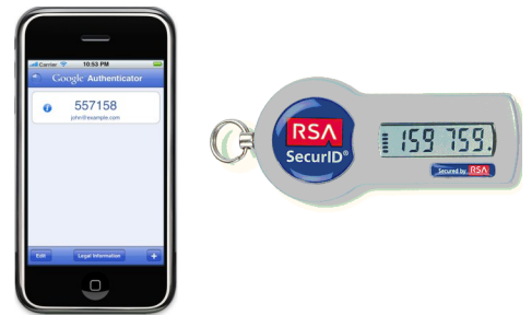
Figure 4.2: The Google Authenticator app is one popular example of a one-time password scheme using pseudorandom functions. Another example is RSA's SecurID token.
